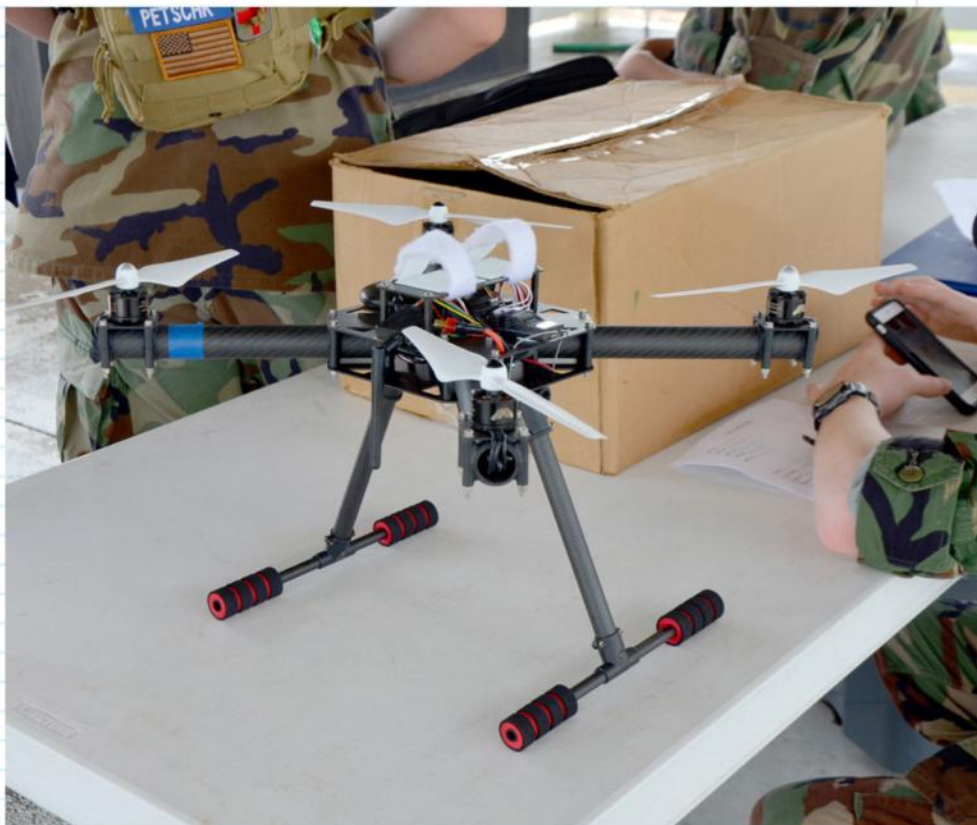
All UAS4STEM competition teams receive a box that contains the components to make the Quadzilla, shown above.
